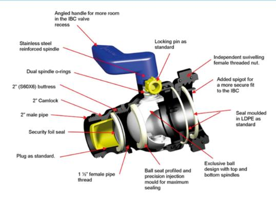
Main features of these **2" full flow Ball Valves** is the unique swivelling back nut which allows for any orientation.
